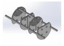
3. Slide Baffle-Spine assembly onto open ends of Copper Tubes
