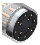
9. Align End Cap 1 concentrically on top of Gasket 1.
