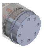
10. Insert Bolts (13) with Washers (15) into End Cap 1 and tighten to 9ft-lbs.
