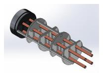
4. Affix other end of Copper Tubes to second Inner End Cap (3-2); Allow to cure for 24 hours.
