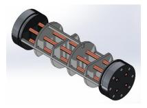
5. Place O-Ring in groove on first Inner End Cap.
