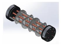
6. Slide assembly, empty groove first, into Shell (16) until empty groove is exposed from far end of Shell. Align inner assembly such that hole is opposite to the flat side of the nearest Baffle.
