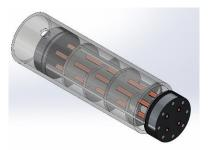
7. Place O-Ring in groove on second Inner End Cap (11-2); Slide assembly backward until Inner End Caps are flush with Shell.
